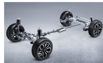
Rear Suspension Type Multiple link independent suspension
